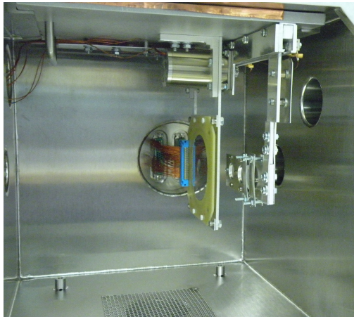
Figure 3: Interior of TPOL vacuum chamber with SSD and production target ladder assembly (from beam left).
