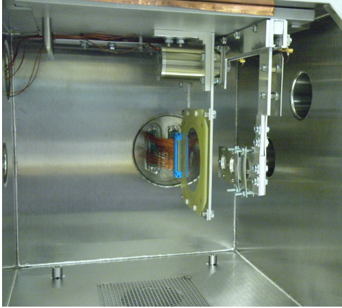
Figure 8: Interior of TPOL vacuum chamber with SSD and production target ladder assembly (from beam left).
