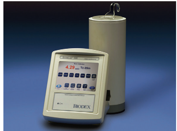
FIGURE 12-17 An ionization chamber dose calibrator. Samples are inserted into the well in the sealed ionization chamber. The current is measured and displayed on a digital readout. (Courtesy Biodex Medical Systems, Shirley, NY.)
