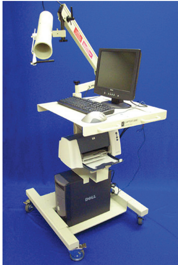
FIGURE 12-19 Typical NaI(Tl) probe system for measuring thyroid uptake of radioactive iodine. (Courtesy Capintec, Inc., Ramsey, NJ.)
