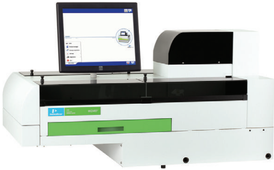
FIGURE 12-7 A NaI(Tl) well counter with automated sample-changing capabilities. Hundreds of samples can be loaded and measured in a single run. This system also incorporates a multichannel analyzer for spectral analysis. (Courtesy PerkinElmer, Inc. Waltham, MA.)
