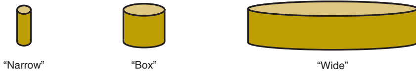
FIGURE 11-7 Examples of detector profiles with different complications for the computation of total detection efficiency.
