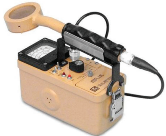
FIGURE 7-11 Radiation survey meter with an external Geiger-Müller (GM) “pancake” counter radiation detector attachment. In addition to the external detector shown, some units have built-in GM counters. (Courtesy Ludlum Measurements, Inc. Sweetwater, TX.)
