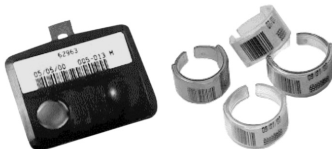
FIGURE 23-3 Examples of personnel dosimeter badges. Left , Thermoluminescent dosimeter (TLD) badge, which usually contains several TLD chips, with one chip being exposed through a thin Mylar window in the badge to permit measurement of low-energy beta radiation. Right , Photograph of ring dosimeters that contain a single lithium fluoride TLD chip and are useful for measuring the dose to the skin and hands from the handling of radionuclides. Bar codes are used on most personnel monitors to permit easy identification and data logging when reading out the TLD chips. (Courtesy Mirion Technologies, Irvine, CA.)
