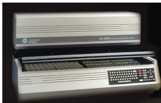
FIGURE 12-16 A liquid scintillation counter with automated sample loading can efficiently count and analyze hundreds of samples. (Courtesy Beckman Coulter, Inc., Brea, CA.)
