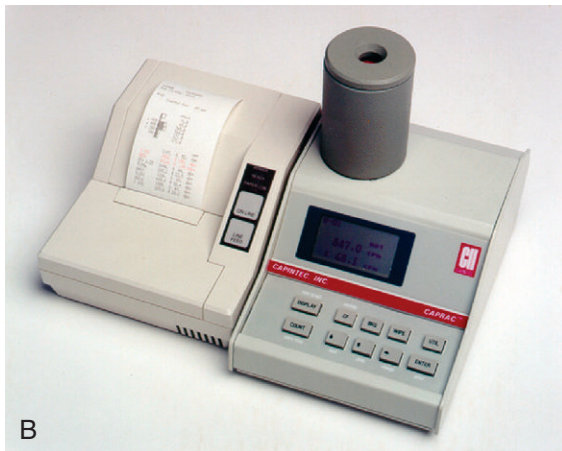
FIGURE 12-1 A, Cross-sectional view of a well-counter detector containing a radioactive sample. B, Photograph of a manually loaded well counter with a digital readout and printer output. (Courtesy Capintec, Inc., Ramsey, NJ.)
