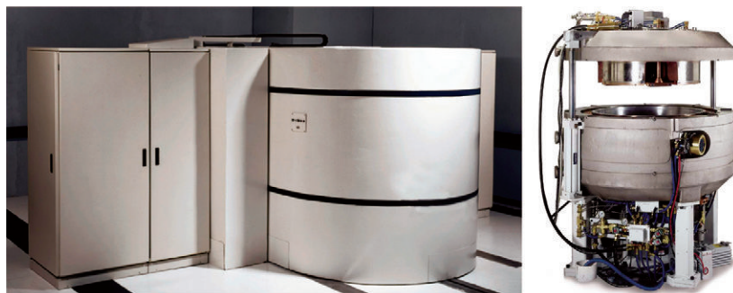
FIGURE 5-5 Photograph of a negative-ion biomedical cyclotron. Left , Cyclotron within concrete shield. Right , The cyclotron itself. (Courtesy Siemens Molecular Imaging Inc., Knoxville, TN.)
