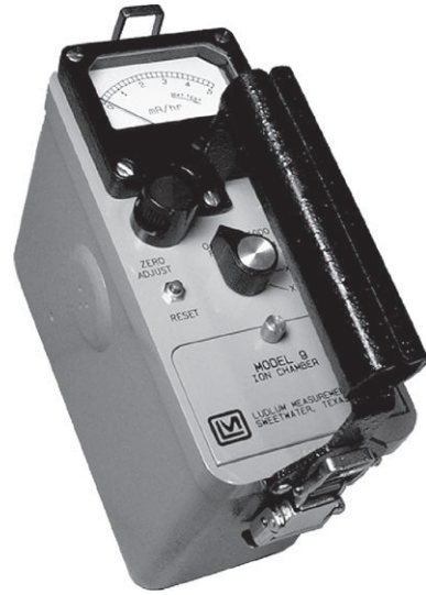
FIGURE 7-3 A battery-powered radiation survey meter. An ionization chamber is contained in the base of the unit, with the entrance window on the bottom face of the device (not shown). The meter indicates radiation level. The rotary switch is used to select different scale factors. (Courtesy Ludlum Measurements, Inc., Sweetwater, TX.)
