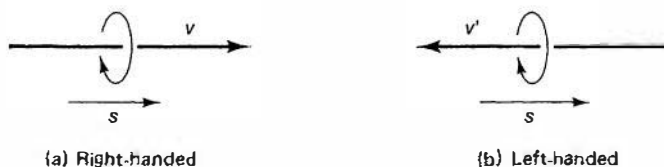
Fig. 4.9 Helicity. In (a) the spin and velocity are parallel (helicity +1 ); in (b) they are antiparallel (helicity -1 ).
