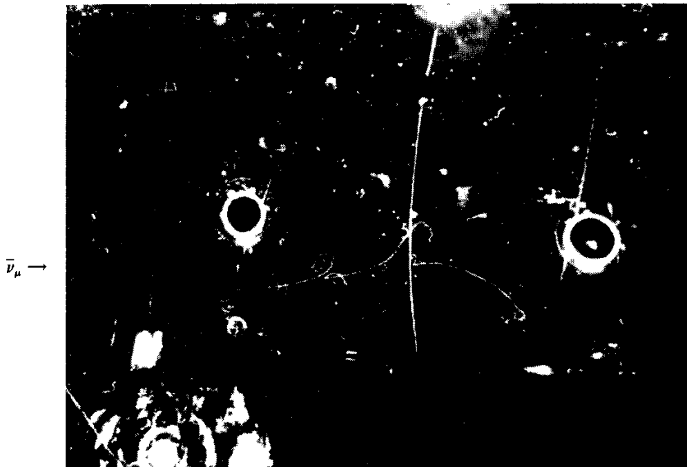
Figure 10.6 The first picture of a neutral weak process ( \bar{\nu}_\mu + e^- \rightarrow \bar{\nu}_\mu + e^- ). The neutrino enters from the left (leaving no track), and strikes an electron, which moves off horizontally to the right, emitting two photons (which show up in the picture only when they subsequently produce electron-positron pairs) as it slows down and spirals inward in the superimposed magnetic field. (Photo courtesy CERN.)
