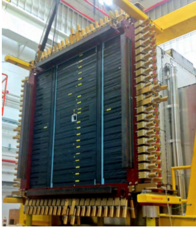
Figure 2.15: Photograph of TOF showing the horizontal paddles and location of the PMTs.
