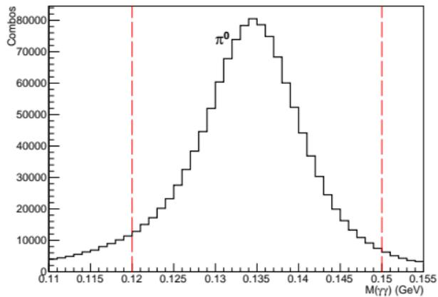
Invariant mass of  $\gamma\gamma$  with red vertical lines indicating the used cut for the selection of  $\pi^0$  from  $0.12 < M(\gamma\gamma) < 0.155$  GeV.
