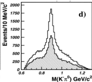
E852  $K^\pm \pi^0$  invariant mass distributions, left, to be compared to 2018 above. E852 shaded distributions have a  $|t| > 0.1 \text{ GeV}^2$  cut applied.
