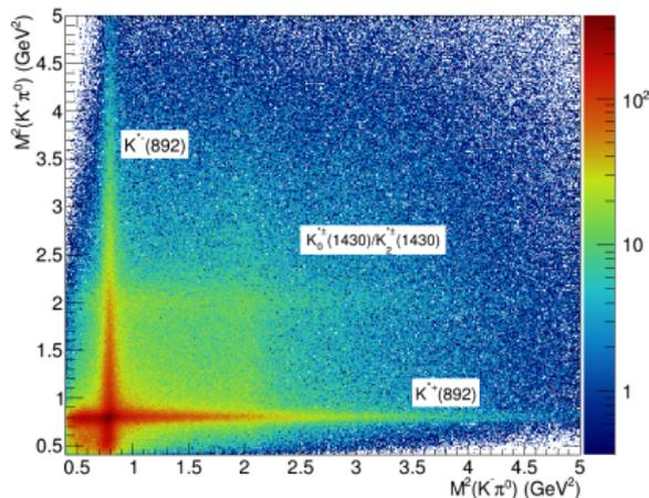
Dalitz of  $M^2(K^+\pi^0)$  vs.  $M^2(K^-\pi^0)$  showing horizontal band for  $K^{*+}(892)$  and vertical band for  $K^{*-}(892)$ , as well as higher mass  $K^*$  states. These are selected from  $0.84 < M(K^{*\pm}) < 0.94$  GeV.
