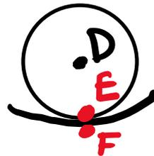
$$\left. \begin{aligned} \vec{v}_D &= \vec{v}_{D/E} + \vec{v}_E \\ \vec{v}_E &= \vec{v}_{E/F} + \vec{v}_F \end{aligned} \right\} \text{But } v_F = 0 \text{ \& } v_{E/F}$$
