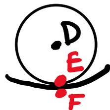
$$\left. \begin{aligned} \vec{v}_D &= \vec{v}_{D/E} + \vec{v}_E \\ \& \vec{v}_E &= \vec{v}_{E/F} + \vec{v}_F \end{aligned} \right\} \begin{array}{l} \text{But } v_F = 0 \\ \& v_{E/F} = 0 \end{array}$$
