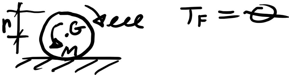
Example: Disk rolling w/out slipping while brake is applied. The brake provides a constant moment (torque)  $M$ . Find distance for the kinetic energy of the disk to go from  $T_I$  to zero
