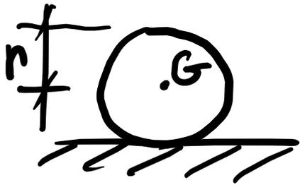
Example: Disk rolling w/out slipping while brake is applied. The brake provides a constant moment (torque)  $M$ . Find distance for the kinetic energy of the disk to go from  $T_I$  to zero
