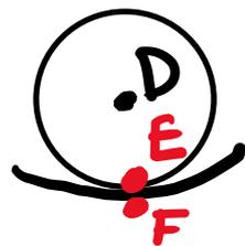
$$\left. \begin{aligned} \vec{v}_D &= \vec{v}_{D/E} + \vec{v}_E \\ \vec{v}_E &= \vec{v}_{E/F} + \vec{v}_F \end{aligned} \right\} \begin{array}{l} \text{But } v_E = 0 \\ \text{ \& } v_F = 0 \end{array}$$
