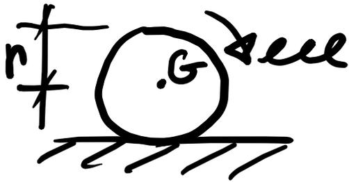
Example: Disk rolling w/out slipping while brake is applied. The brake provides a constant moment (torque)  $M$ . Find distance for the kinetic energy of the disk to go from  $T_I$  to zero
