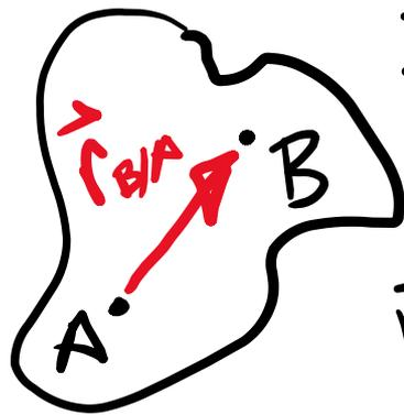
If points A & B are on a rigid body in plane motion
