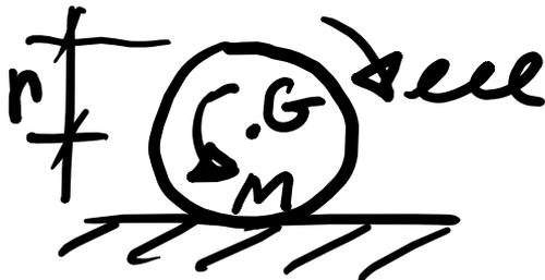
$T_F = 0 \quad \& \quad \int_{\theta_I=0}^{\theta_F} M d\theta = -M\theta_F$
