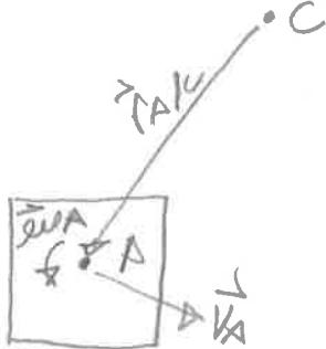
For point A we could find some other point C such that  $\vec{v}_A = \vec{\omega}_A \times \vec{r}_{AC}$
