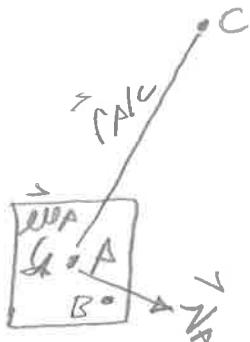
$$\begin{aligned} \text{we have } \vec{v}_A &= \vec{\omega}_A \times \vec{r}_{AC} \text{ & want} \\ \text{to construct } \vec{v}_B: \quad \vec{v}_B &= \vec{v}_{Ba} + \vec{v}_A \\ &= \vec{\omega}_A \times \vec{r}_{Ba} + \vec{\omega}_A \times \vec{r}_{AC} = \vec{\omega}_A \times (\vec{r}_{Ba} + \vec{r}_{AC}) \\ &= \vec{\omega}_A \times (\vec{r}_B - \vec{r}_A + \vec{r}_A - \vec{r}_C) = \vec{\omega}_A \times (\vec{r}_B - \vec{r}_C) \\ &= \vec{\omega}_A \times \vec{r}_{BC} \end{aligned}$$
