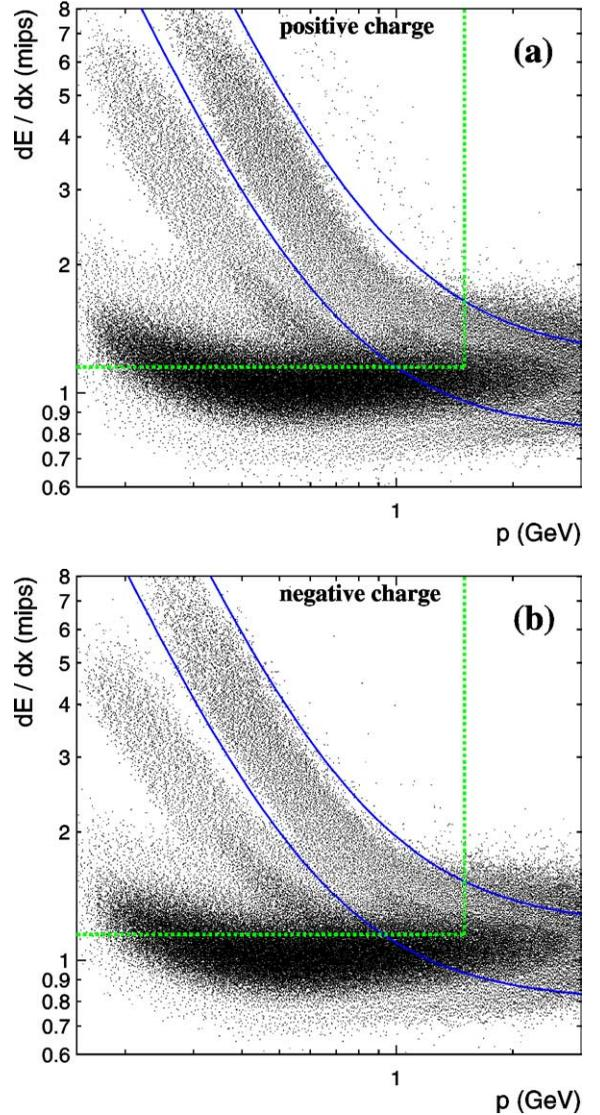
Fig. 2. The  $dE/dx$  distribution as a function of the track momentum for: (a) positive and (b) negative tracks. The  $dE/dx$  is normalised to a minimum ionising particle, defined as the average truncated mean of pion tracks in the momentum range  $0.3 < p < 0.4$  GeV. The solid lines indicate the (anti)proton bands used in this analysis, and the dotted line denotes the cuts  $dE/dx > 1.15$  mips and  $p < 1.5$  GeV.
