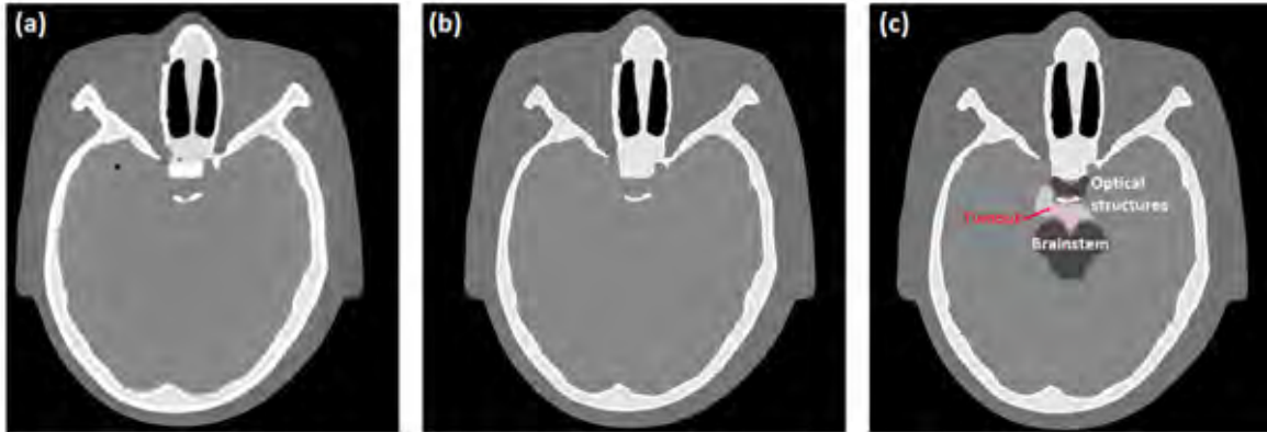
Figure 4.3: (a) xRay CT scan of the physical head phantom; (b) corresponding image of the HighResHead; (c) same image of the modified version of HighResHead with tumour and surrounding OAR.
