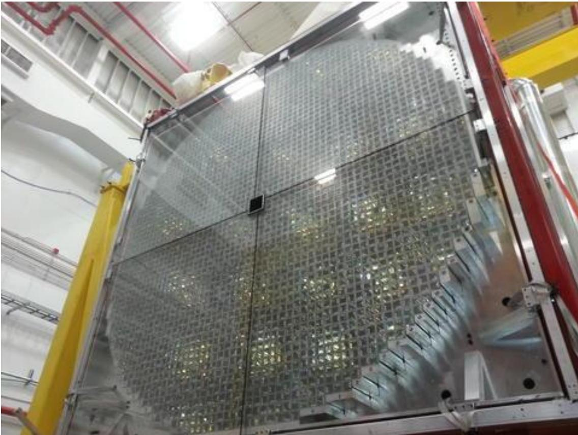
**Figure 2.16:** Fully constructed FCAL with 2800 lead blocks exposed.
