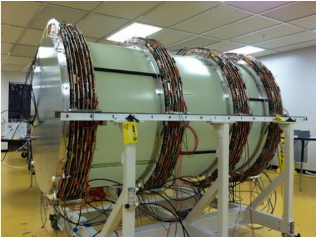
**Figure 2.12:** Fully constructed FDC shown outside of the superconducting solenoid magnet.
