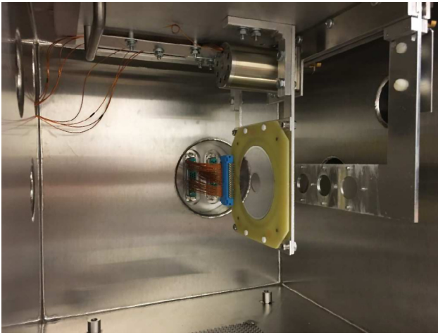
Fig. 12. (Color online) Interior view of vacuum chamber, with detachable plate, converter tray positioning system and silicon strip detector installed. See Fig. 10 for details of the detector plate assembly.
